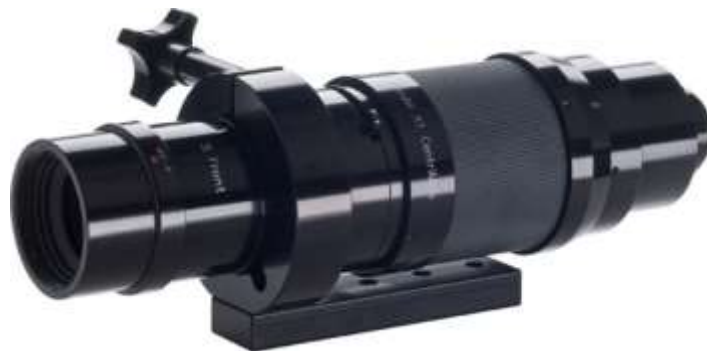
Figure 4. An example of a long distance microscope that was considered. This particular model theoretically satisfied technical requirements, but was over $3,000.
